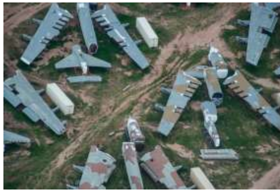
B-52 Stratofortress bombers are dismantled in accordance with the Strategic Arms Reduction Treaty at the 309th Aerospace Maintenance and Regeneration Group's Aircraft and Missile Storage and Maintenance Facility on Davis-Monthan Air Force Base, Ariz., in 2017. Each of the 365 B-52s were flown to the AMARG facility in the early 90s and cut into five pieces in accordance with the treaty
